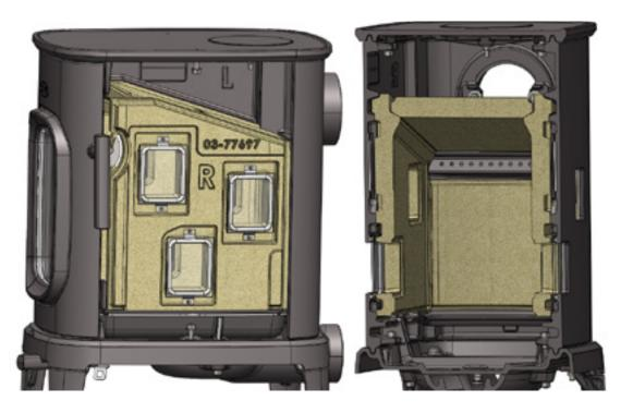
The air regulation on the SAGA 107 has Air Pockets around the side windows and Air Flow over the glass, to keep them as clean as possible, so they do not have to be cleaned regularly.
